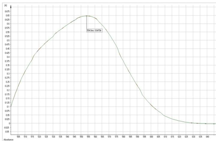
Figure 1. Wavelength Maximum Results The reaction of borax and Curcumin.
